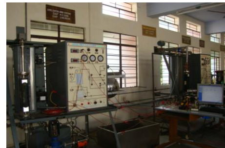
Figure 1: Experimental Setup of a Coupled Tank level system
