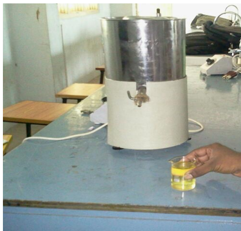
Viscometer for finding the viscosity of oil
