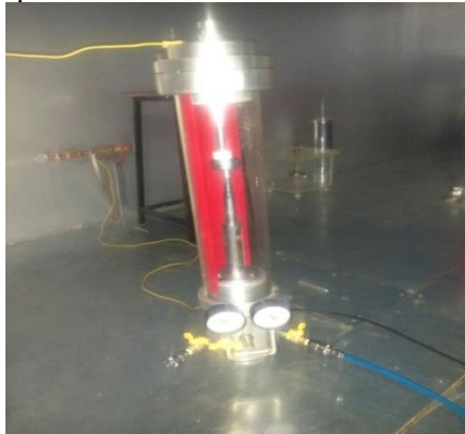
Figure 1: Gas chamber to house the Electrodes, filled with gas and maintain at different pressures.
