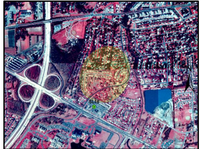
Figure 2. Sampling footprint layout shown overlaid on a GIS map of the sampling location. Footprint shows majority of emissions affecting a local neighborhood.
