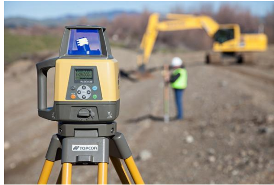
Figure 3. Laser level installed in the Field (Topcon, 2020) https://www.topconlaser.com.au/accuracy_laser_levels
