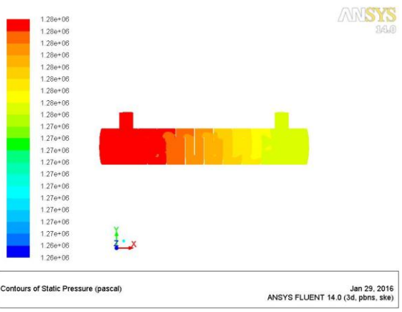
Fig. 8 Contours of Shell Side Fluid's Pressure of Shell and Tube Heat Exchanger with Segmented Baffles
