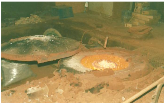
Figure 1: An opened diesel fired furnace after melting Aluminium and bringing it to its pouring temperature
