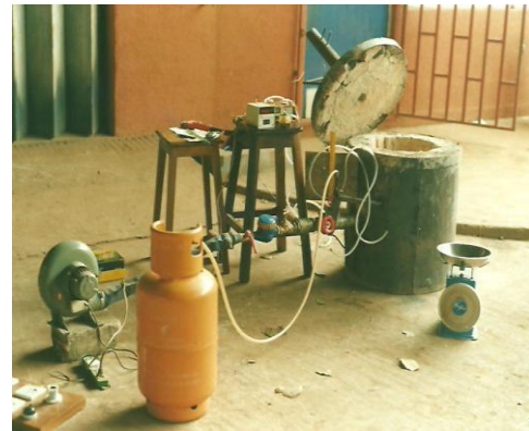
Figure 2: An opened butane gas fired furnace after melting Aluminium and bringing it to its pouring temperature
