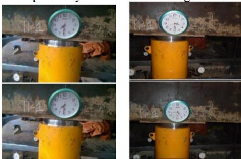
Fig. 10. Pile head displacement meter.
