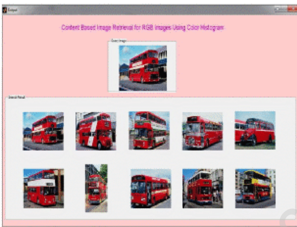
Fig 5 Retrieval results for red bus query image with k = 10 and Bhattacharyya distance
