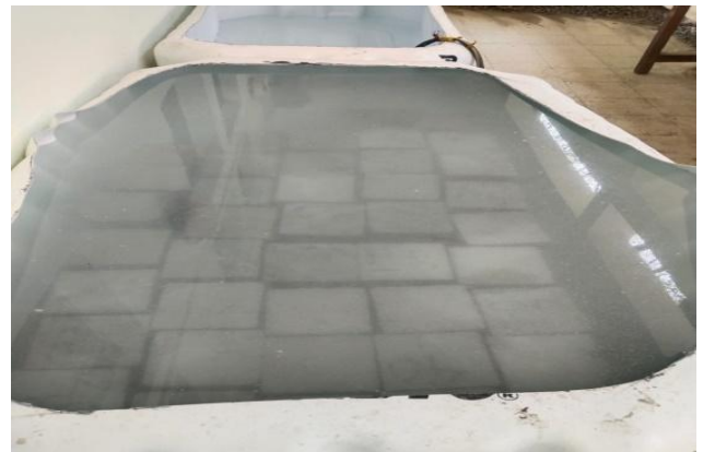
Figure 3: Curing in leachate
