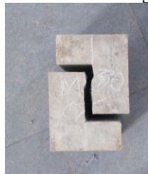
Fig.5: Failed push-off specimen
