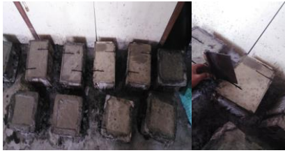
Fig.4: Cubes and push-off shear strength specimens
