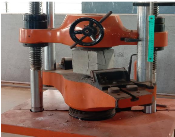
Fig 3 compressive strength test
