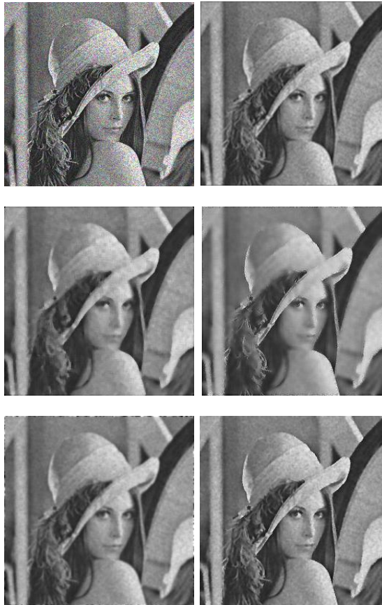
Figure: 1.a Speckle Noise Added Image, 1.b Applying Mean Filter, 1.c Applying Median Filter, 1.d Applying Wiener Filter, 1.e Applying HE, 1.f Applying PME.
