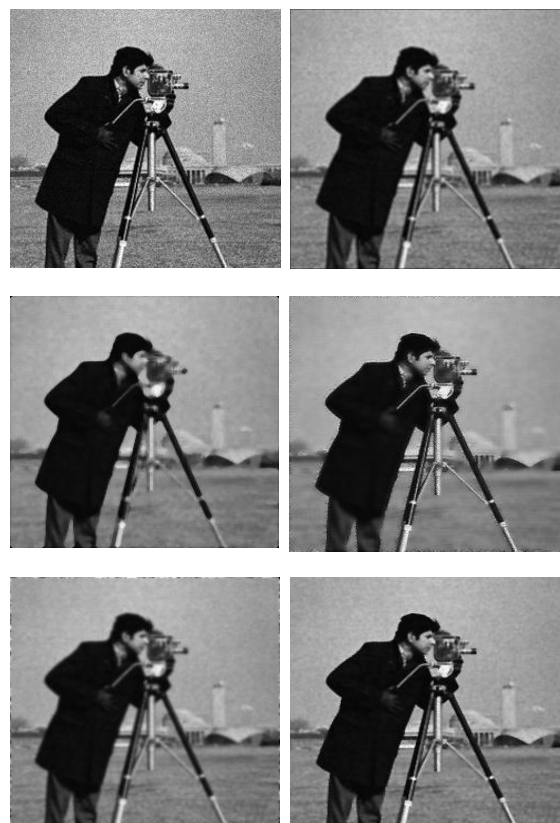
Figure: 4.a Poisson Noise Added Image, 4.b Applying Mean Filter, 4.c Applying Median Filter, 4.d Applying Wiener Filter, 4.e Applying HE, 4.f Applying PME.
