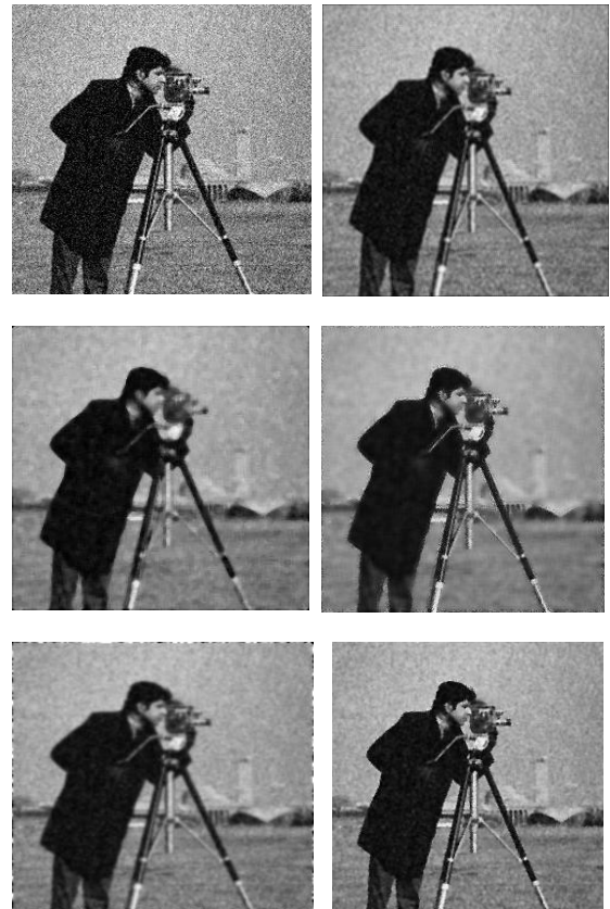
Figure: 2.a Gaussian Noise Added Image, 2.b Applying Mean Filter, 2.c Applying Median Filter, 2.d Applying Wiener Filter, 2.e Applying HE, 2.f Applying PME.
