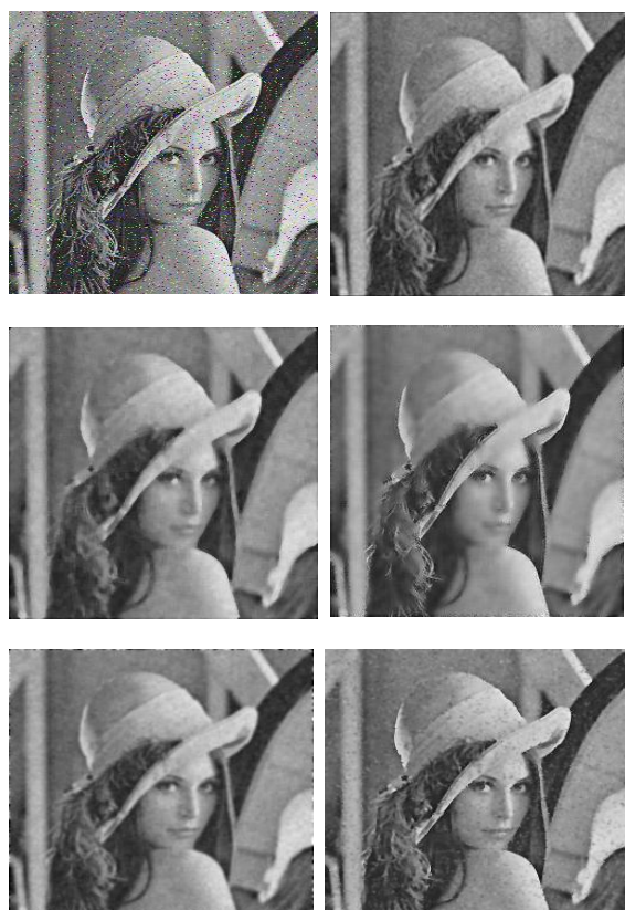
Figure: 3.a Salt and Pepper Noise Added Image, 3.b Applying Mean Filter, 3.c Applying Median Filter, 3.d Applying Wiener Filter, 3.e Applying HE, 3.f Applying PME.
