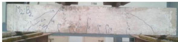
Figure 3: Cracking Pattern of Beam B2/M25/AST1/NF
