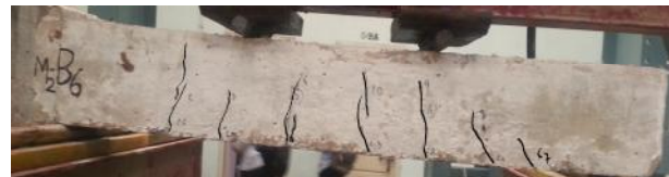
Figure 7: Cracking Pattern of Beam B6/M25/AST1/WF/1.5%
