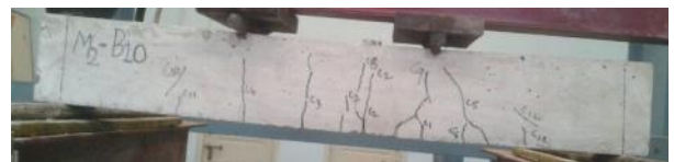
Figure 11: Cracking Pattern of Beam B10/M50/AST1/NF
