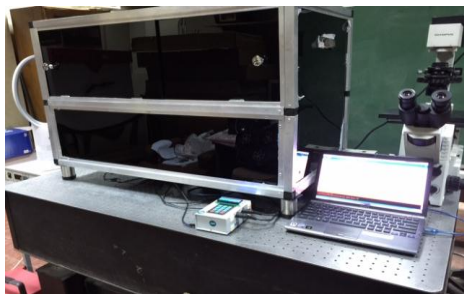
Figure 0-1 Our complete confocal microscopy system CLSM with AY128-R microcontroller. This system is composed of inverted microscope, confocal part including scan head, laser optics, and computer.
