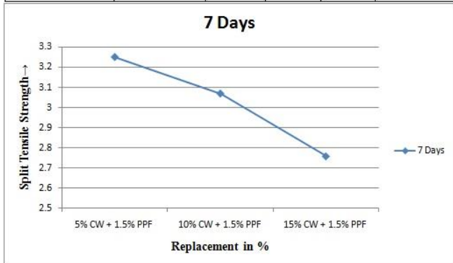
Fig 6- Split Tensile Strength Graph for Replacement of cement by ceramic waste along with addition of PPF.
