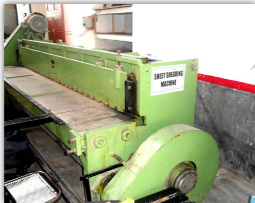
Fig.12 Power sheet shearing machine, Central workshop, NIT Srinagar
