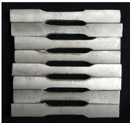
Fig.7 Tensile Specimens from Welding Piece
