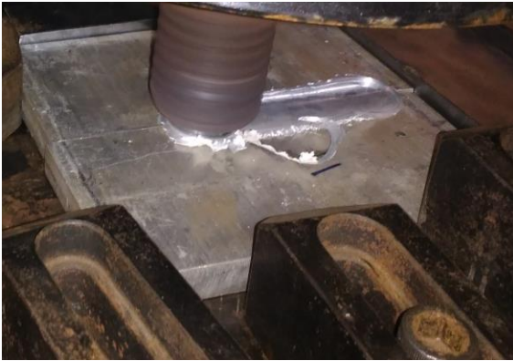
Fig. 6 Weld specimens on FSW Machine
