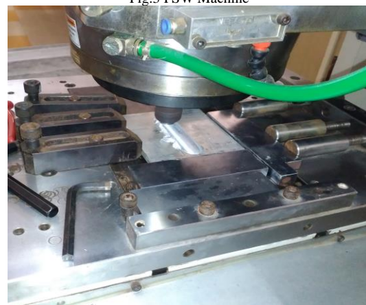
Fig. 4 FSW experimental set up
