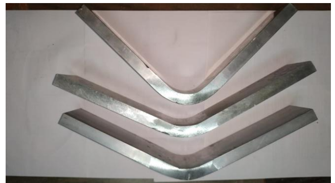
Figure 11: sample weldments after bend test
