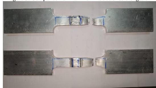
Figure 6: samples in Tensile testing showing fracture in HAZ area
