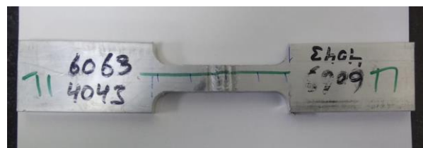
Figure 3: Weld sample prepared for tensile test
