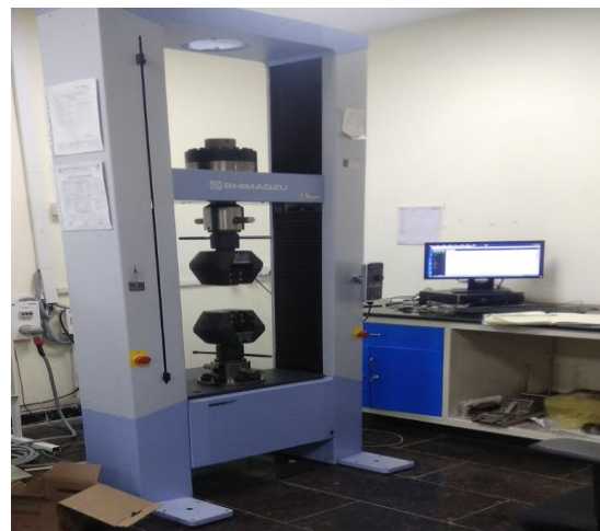
Figure 7: 300kN capacity SHIMADZU UTM
