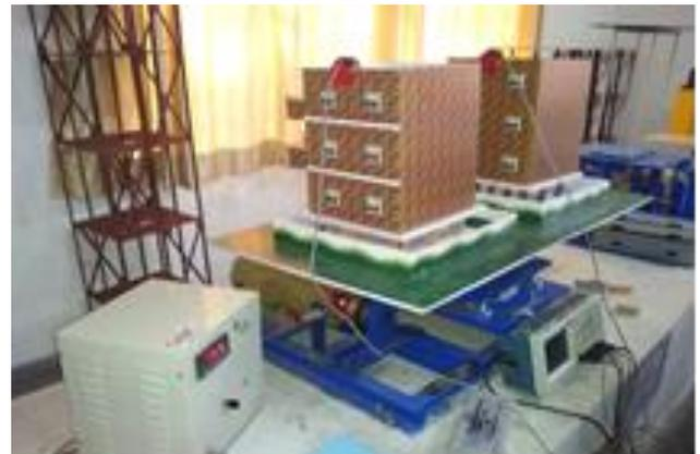
The experimental setup consists of shake table, RPM machine, Accelerometer1 and Accelerometer 2, computer. When the shake table starts giving motion then displacement and acceleration waves are readings are automatically taken by software of computer. In this figure Accelerometer 1 is attached to spring base building and Accelerometer 2 is attached to fixed base building. The software gives accurate reading at small waves also.
