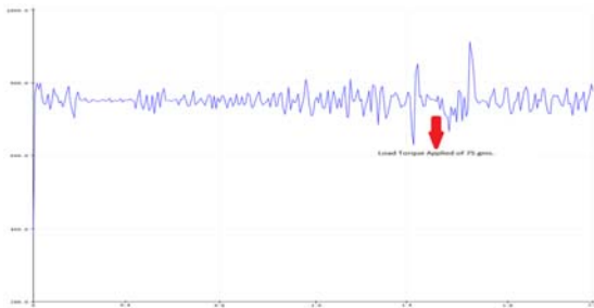
Fig. 19. Hardware based speed response of BLDC motor drive at 750 rpm using PI controller
