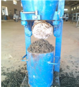
Figure (3) Compaction factor test
