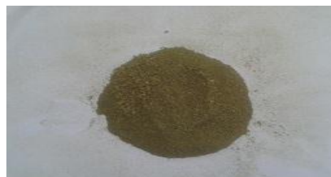
Fig. 3. Neem leaf powder average particle size 72 \mu\text{m}
