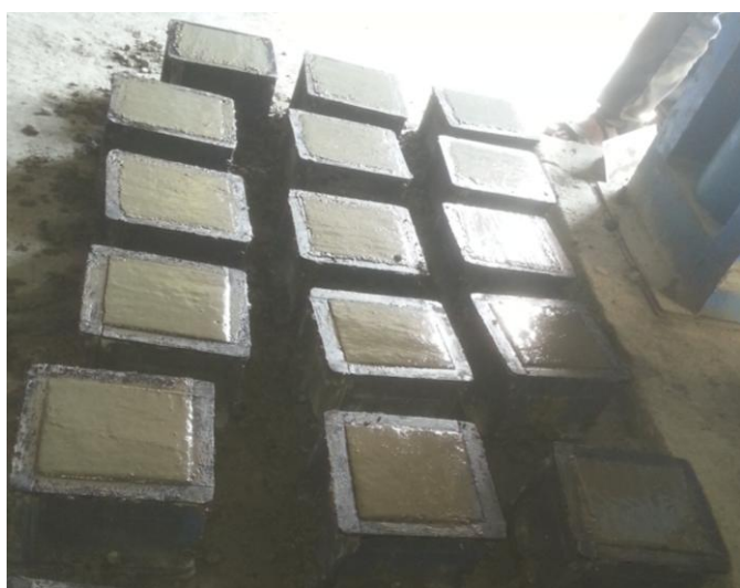
Fig. 1 casting of cubes
