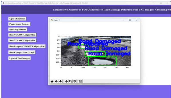
Fig 2: YOLOv8 detection output illustrating multiple detected damage regions.
