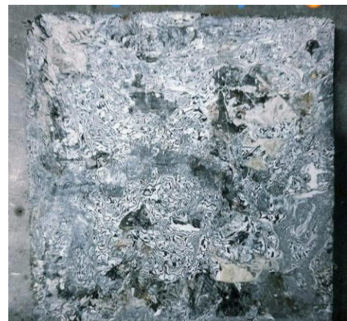
Figure 2: Final LDPE Tile
