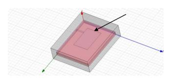
CaseII Rectangular Microstrip Patch Antenna DESIGN (Contacting Feed Line)
