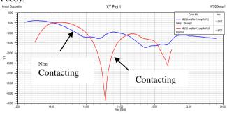
The above plot is extensively representing the combined Rectangular plots for both the antennas The red line plot is for contacting feed line and the blue is for Non Contacting feed line. The highest return loss that we are obtaining is of -44db.
