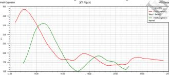
The above plot is representing the superimposed VSWR Plot for capacitive and Non Capacitive coupled feed. The Green Line curve variation is representing the plot for Contacting feed line and the Red curve is representing the plot for Non Capacitive coupled feed.
