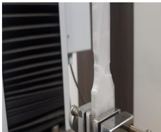
Figure 7- Specimen clamped in the UTM
