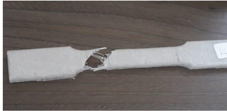
Figure 8- Elongated PLA material part no 21
