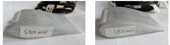
Fig. 7. Wooden models of S819 and S 821 airfoil.
