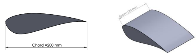
Fig. 4. 2D and 3D cad representation of S821 airfoil.
