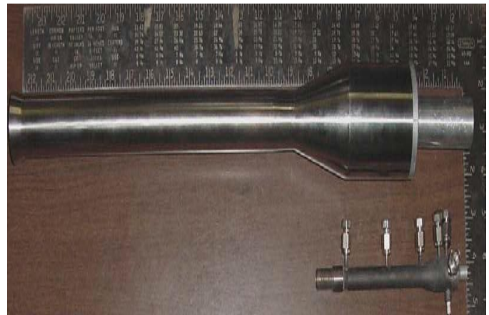
Fig.1. 3:10 scale down of the Bailey Machine Services (BMS) hobby-scale pulsejet
