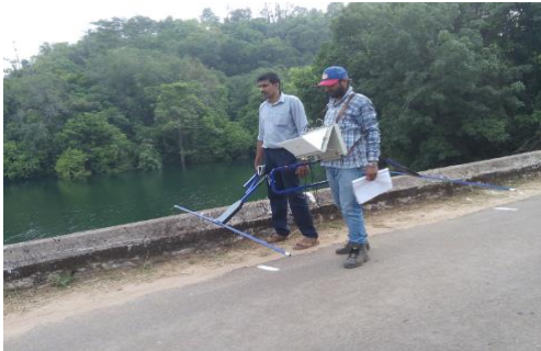
Fig.5. GPR test on peruvannamuzhi earth dam
