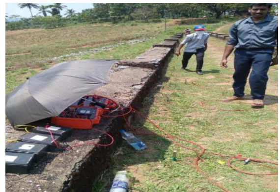
Fig.7. Data acquisition of ERT method
