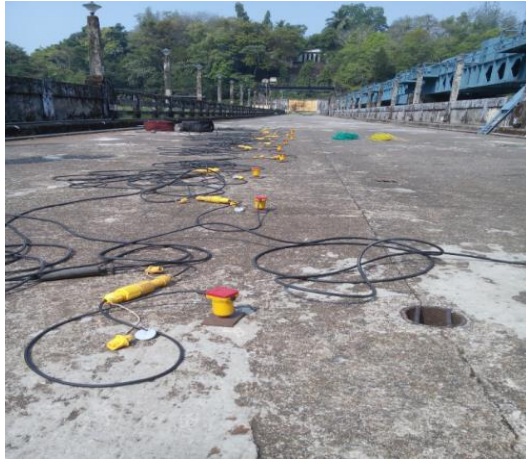
Fig.8. Data acquisition of ReMi method
