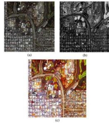
Fig 3: IKONOS data set. (a) Natural color composite of the first three bands, (b) the corresponding NIR channel, and (c) the fusion result.
