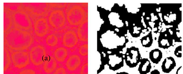
Fig. 5. Result of thresholding in LAB color space. (a) The image in LAB color space, (b) the same image after thresholding
