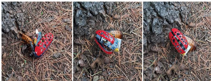
Fig.2. Cyborg insect locomotion assistance using bio-inspired 3Dprinted artificial limb [1]
