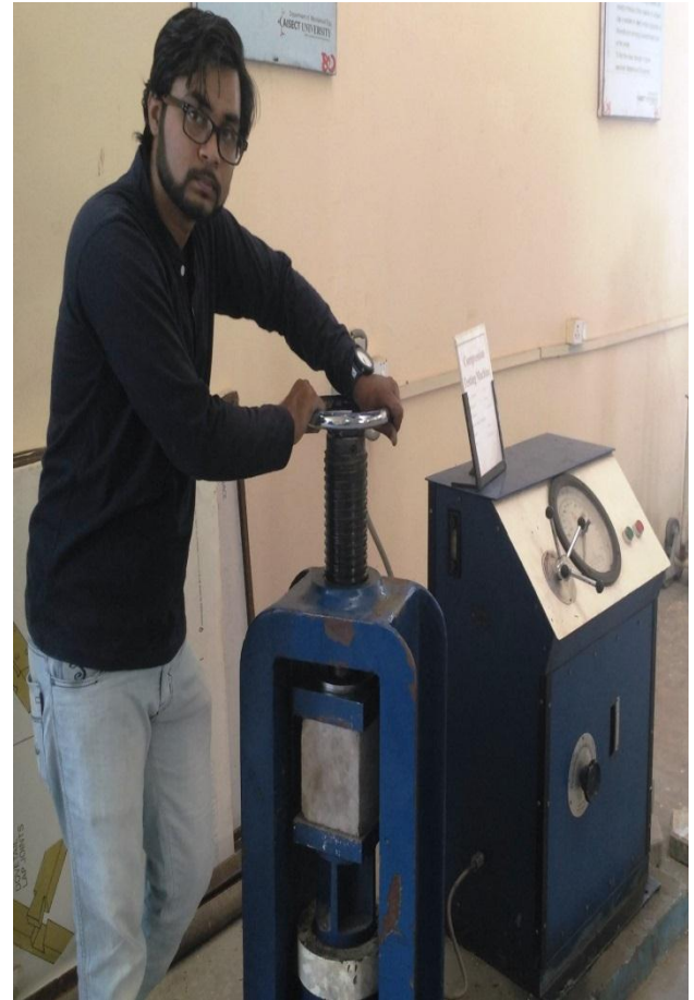
Fig 10 Compressive Strength of Conventional Concrete Cubes
