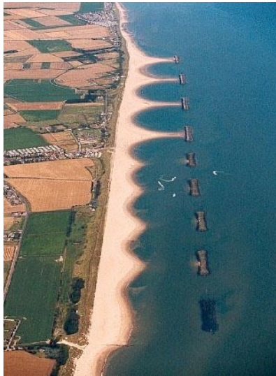
Fig 7: Offshore detached breakwater
