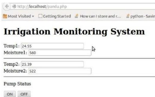
Fig 7, Web page displaying temperature and moisture data with pump status
