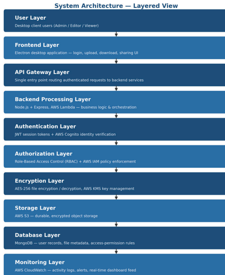
Fig. 1. SecureVault's ten-layer architecture, from the user-facing client down to storage and observability.
