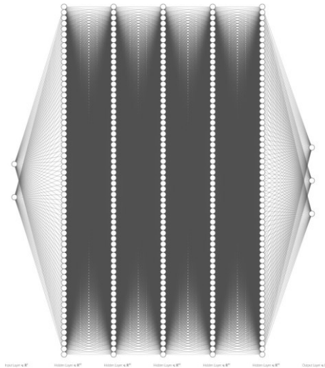
Fig.2: Neural Network schematic for the PINN, contains 2 input neurons, 5 hidden layers, each with 64 neurons each, and 1 output layer with 3 neurons. In the input layer, the spatial coordinates x and y are represented as neurons. In the next 5 hidden layers, each with 64 neurons are responsible for capturing and learning the complex relationships and features within the fluid flow data. In the output layer, the velocity components in the x and y directions are received along with the pressure.
