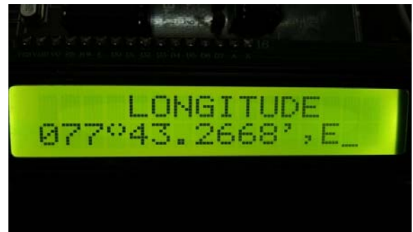
Fig.6 LCD displaying longitude value of child.
