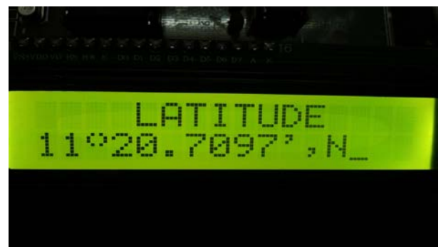
Fig.7 LCD displaying latitude value of the child.
