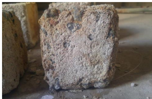
Fig 2. QBBSCC of w/b ratio 0.4 after immersion in 5% H 2 SO 4 Solution for 180 days
