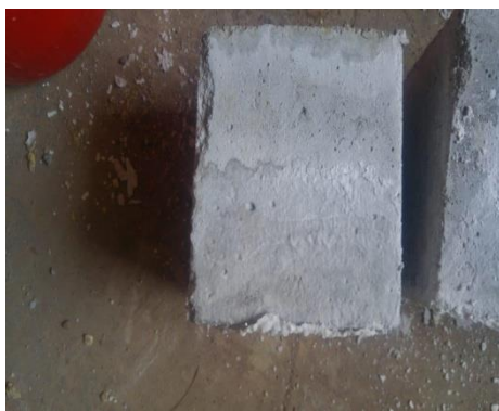
Fig 6. QBBSCC of w/b ratio 0.4 after immersion in 5% Na 2 SO 4 solution for 180 days
