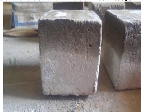
Fig 3. QBBSCC of w/b ratio 0.3 after immersion in 5% HCl Solution for 180 days
