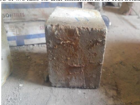
Fig 4. QBBSCC of w/b ratio 0.4 after immersion in 5% HCl Solution for 180 days
