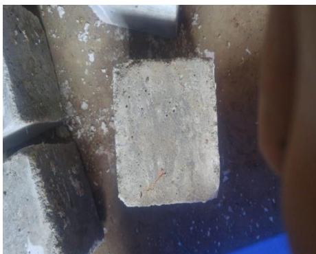
Fig 5. QBBSCC of w/b ratio 0.3 after immersion in 5% Na 2 SO 4 solution for 180 days
