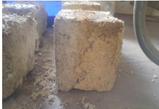
Fig 1. QBBSCC of w/b ratio 0.3 after immersion in 5% H 2 SO 4 Solution for 180 days
