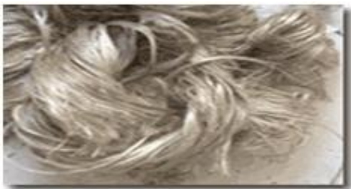
Fig 5 Jute fiber obtained from stem of Jute plant
