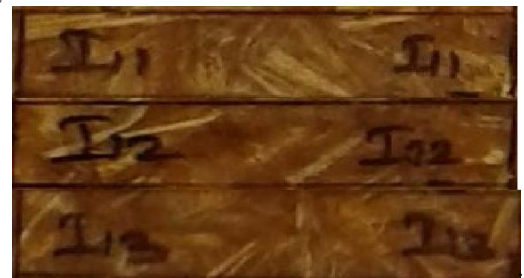
Figure 4.3 Impact test specimen of pineapple leaf fibre
