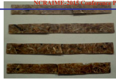
Fig 5.2: specimen after tensile test
