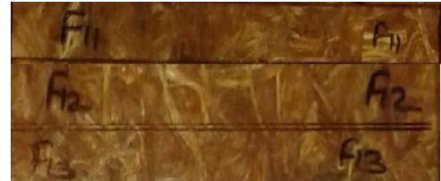
fig 4.2 Flexural test specimen of pineapple leaf fibre
