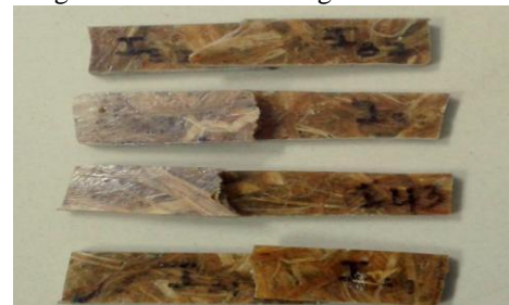
Fig.5.3 Specimens after impact testing
