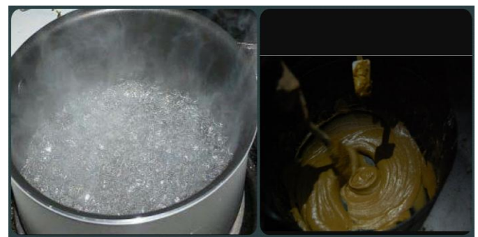
Fig 3 Bentonite treating with 2.5% Na 2 CO 3
