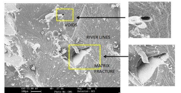
Fig.6 (c): SEM image of hybrid composite with 3 wt% extracted residue powder and 5 wt% CFF in epoxy resin at 100X magnification
