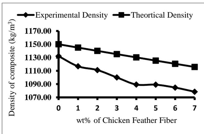
Fig. 2: Effect of wt% of CFF on density of composite
