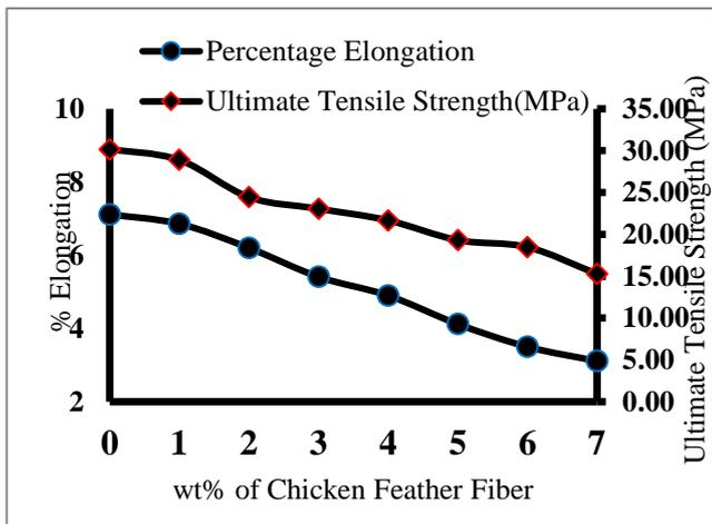
Fig. 3: Effect of CFF wt% on ultimate tensile strength (MPa) and percentage elongation in epoxy resin based composite
