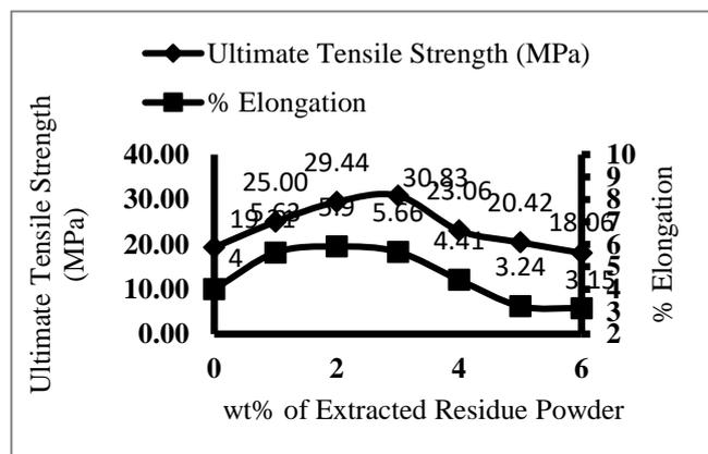
Fig. 4: Effect of ERP wt% (with 5wt% CFF) on ultimate tensile strength and percentage elongation on hybrid composite
