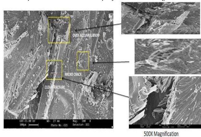
Fig.6 (f): SEM image of hybrid composite with 6 wt% extracted residue powder and 5 wt% CFF in epoxy resin at 100X magnification
