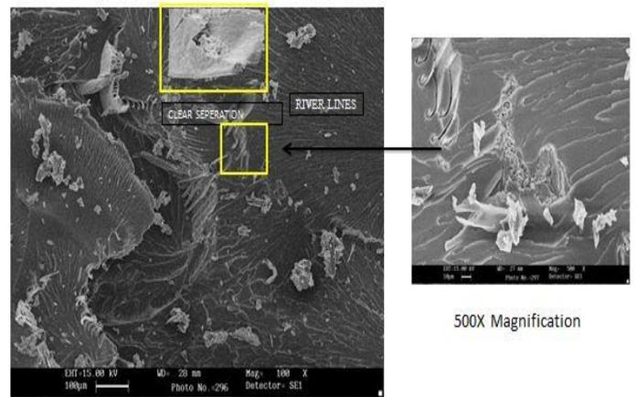
Fig.6 (a): SEM image of hybrid composite with 1 wt% extracted residue powder and 5 wt% CFF in epoxy resin at 100X magnification
