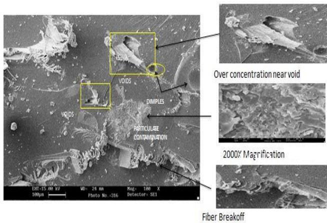
Fig.6 (e): SEM image of hybrid composite with 5 wt% extracted residue powder and 5 wt% CFF in epoxy resin at 100X magnification
