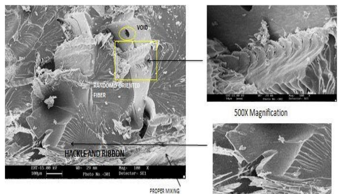
Fig.6 (b): SEM image of hybrid composite with 2 wt% extracted residue powder and 5 wt% CFF in epoxy resin at 100X magnification
