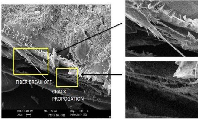
Fig.6 (d): SEM image of hybrid composite with 4 wt% extracted residue powder and 5 wt% CFF in epoxy resin at 100X magnification
