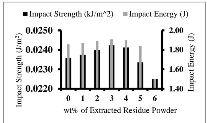
Fig. 5: Effect of ERP wt% (with 5 wt% CFF) on impact strength and impact energy
