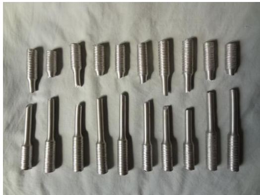
Fig. 2. Tensile test specimens after test
