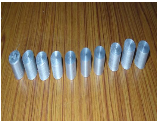
Fig. 3. Brinell Hardness test specimens
