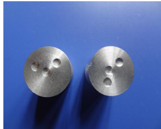
Fig. 4. Brinell Hardness tested specimens
