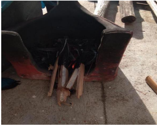
Figure.4. Burning of Bamboo For Getting Ash
