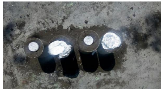
Figure.8. Sample Mould After Casting Process
