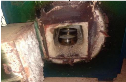
Figure.5. Heat Treatment of Ash in Muffle Furnace
