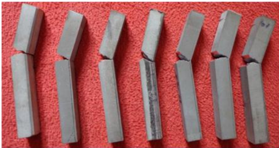
Fig.12 Specimen after conducting Izod Impact Test
