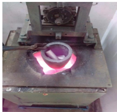
Fig. 3. Loading Al-alloy into the furnace
