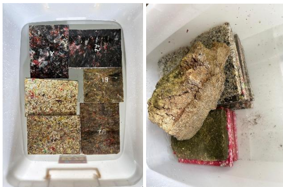
Fig 7. Container and water setup used for thickness swelling test
