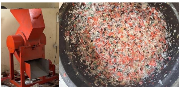
Fig 1. Plastic shredding process
