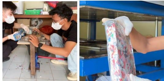
Fig 2. Manual pressing and sealing method and the result
