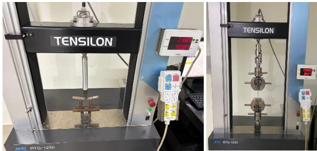
Fig 5. UTM (Universal Testing Machine) for MoR, MoE, tensile strength test
