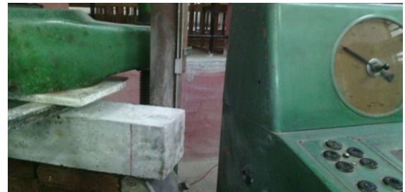
Fig-3; Arrangement for flexural test of beam.
