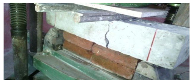
Fig-4; Failed beam
